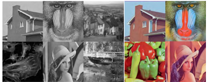
Fig. 7. The standard test images. Left: six standard gray scale images for Gaussian denoising experiments; Right: four standard RGB images for camera raw image simulation.
