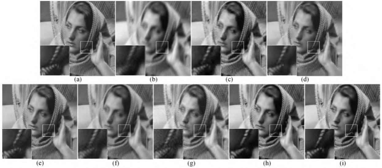
Fig. 9. Deblurring comparison on image “Barbara”. (a) Original image; (b) Noisy and blurred image (Gaussian kernel: 19 \times 19 , \delta_e = 2.25 ); Results by (c) LevinSps (PSNR = 30.14dB; SSIM = 0.885), (d) EPLL (PSNR = 28.21dB; SSIM = 0.904), (e) DMSP (PSNR = 28.78dB; SSIM = 0.897), (f) DPE (PSNR = 30.94dB; SSIM = 0.889), (g) DAEP (PSNR = 28.50dB; SSIM = 0.798), (h) EDAEP (PSNR = 31.83dB; SSIM = 0.910), and (i) MEDAEP (PSNR = 31.88dB ; SSIM = 0.912 ).
